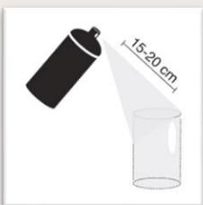
Apply AESUB white from 15-20 cm away. Spray over the entire surface that you will be scanning. Gently push down the spray button and move the can across the area using even, back and forth strokes. Move at a consistent pace without pausing at one point to achieve an even coat. Once the coat is applied, you can scan the object in usual manner. Unlike traditional pigment spray, AESUB white does not contain titanium dioxide suspected of causing cancer through the inhalation route.
