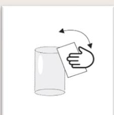
AESUB white is a permanent scanningspray. Coated parts need to be cleaned or disposed after scanning. AESUB white was developed to allow easy cleaning. Utilize a soft brush in combination with water and a towel to clean coated parts.
