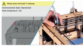
**12.** Next step is to click the top Z-end stop, rotate the build plate screw or click it with your screw driver/finger.
