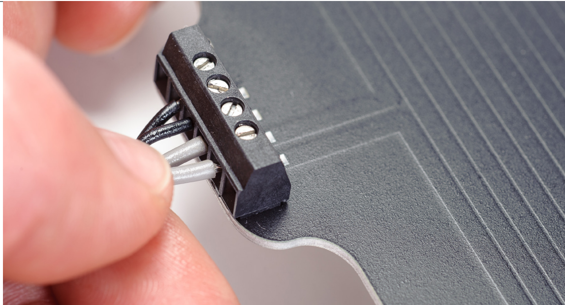
image 76: Connecting the Heated bed Cable.
